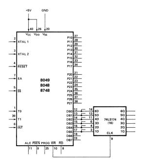
The latch can be loaded with the OUTL instruction. After the latch is loaded the BUS output state can be modified with the ANL BUS, # DATA and the ORL BUS, # DATA. The OUTL generates a WR strobe; ANL and ORL do not. In this configuration DB0-DB7 will be momentarily disturbed while the external latch is loaded.
